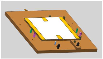
2) Position bottom sensor HV tail (single tail) in its (peach) positioner. Note: The connector should seat inside the precision cut out of the positioner.
