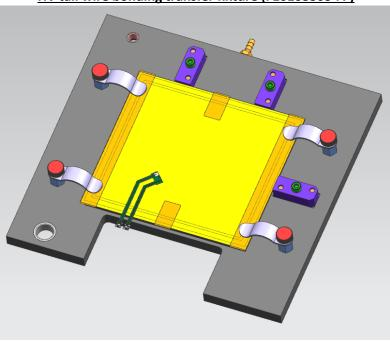
HV tail wire bonding transfer fixture (F10108303-A-)
