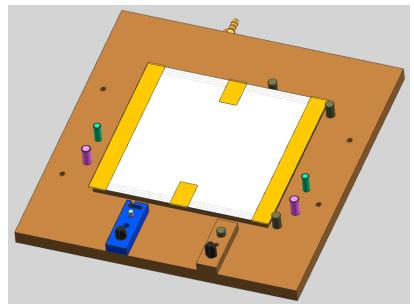
2) Position top sensor HV tail (double tail) in its (blue) positioner.
