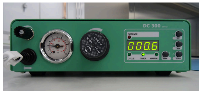
Figure 4: Front panel of a Vieweg DC 300 semi-automatic glue dispenser used in the base plate insert gluing.
